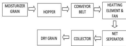
FIG. PROCESS DIAGRAM
